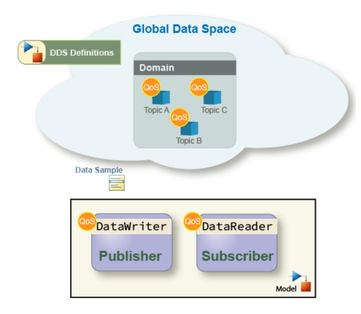
You then configure the DDS interface. The DDS interface is the connection point between the application and the DDS network. Specifically, when you use the DDS Blockset, the interface is the Topic and QoS specified on the DataWriters and DataReaders for your application.
