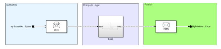
In the Simulink model for the Shapes Demo, view how the DDS blocks, Take DDS Sample and Write DDS Sample, are used to subscribe to and publish the location of the shape.
